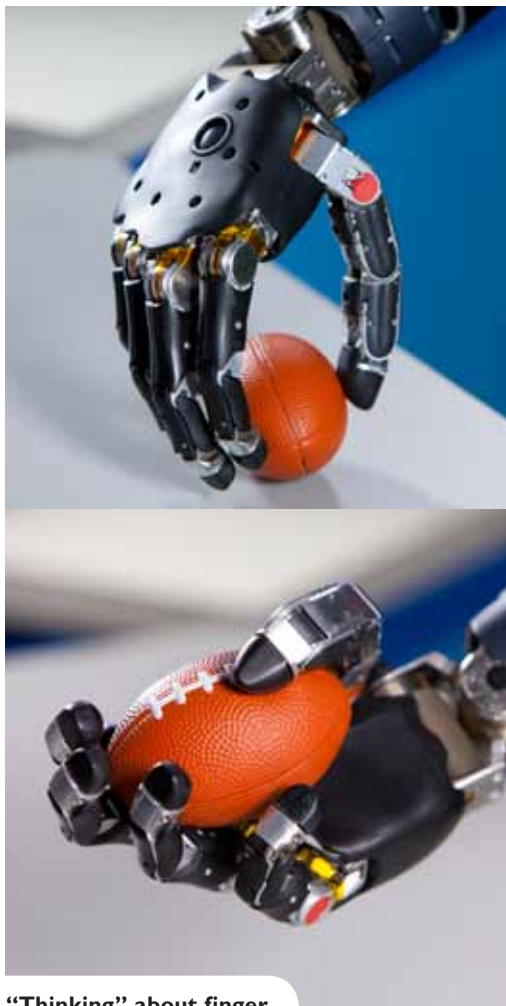
“Thinking” about finger movements caused electrical activity in the brain, which moved the prosthetic digits.
